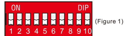
**The 9th Dip Switch:** it is valid when it is configure as sending end. As figure 2, it is the normal mode when OFF, sending out the data from the DMX console; As figure 3, it is the self-testing model when ON, sending out the auto-generated DMX console data(170 pixels full color smooth changing effect).
