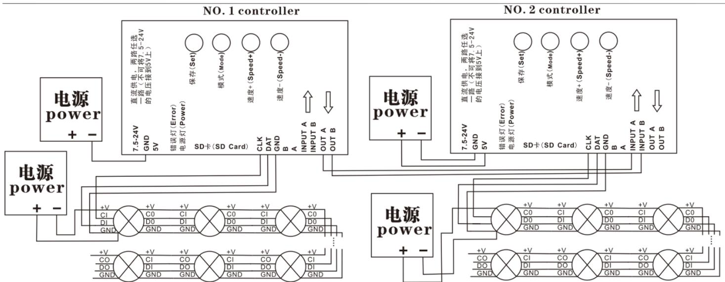
when the controller control less than 512 pixels the frame rate can reach 30fps,
